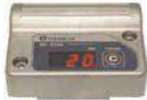
* M-DW shows 20° from snug torque.
